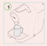
Make sure that the lever is lowered and there is not a capsule inside the capsule compartment.
