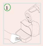
When warning light F is steadily lit in red, The Loop is disabled and the used capsule drawer must be emptied (same procedure as above). Please make sure that you slide the used capsule drawer and drip tray all the way back in to the machine in order for the light F to switch off and The Loop to be re activated.
