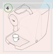
5. Press the correct sized button A, B, or C that was indicated on the top foil cover of the capsule.
